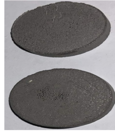
Figure 3. Image of powdered steel after sintering
