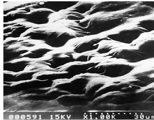
Figure 5. Micrographs of LDPE film with the content of the modifying additive (PFR) 0.05 wt%
