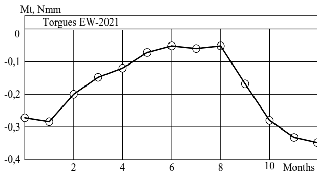
Figure 6. Variation of gravitational torques in 2021 along the latitude of the Earth equal to 50°55'N
