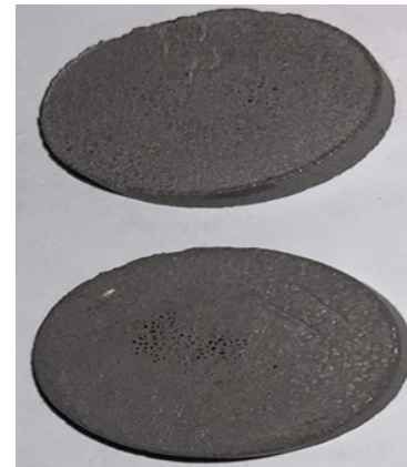
Figure 3. Image of powdered steel after sintering
