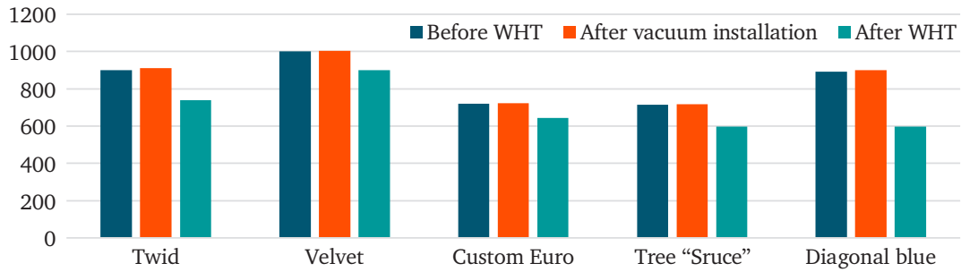
Figure 13. Influence of the existing and developed methods of WHT on the breaking load of the examined samples
