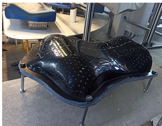
Figure 1. General view of the bottom cushion of the vacuum installation made of composite material Source: compiled by the authors
