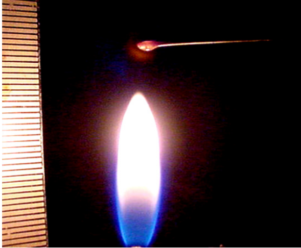
Figure 3. Visualization of the H_2 flame fragment by evaporation of NaCl molecules in a diffusion propane flame from the upper side of the flame
